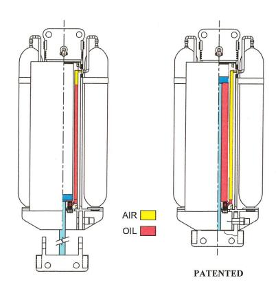
accumulator allowing for a compact design. The port at the lower end also houses a shut off valve. This valve may be closed at any point in the stroke of the DSC hydraulically locking the load for lifting.
